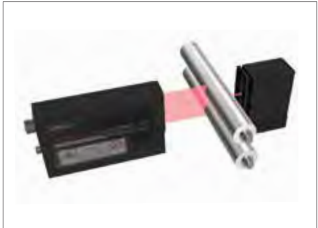
Measurement of gap between rollers
