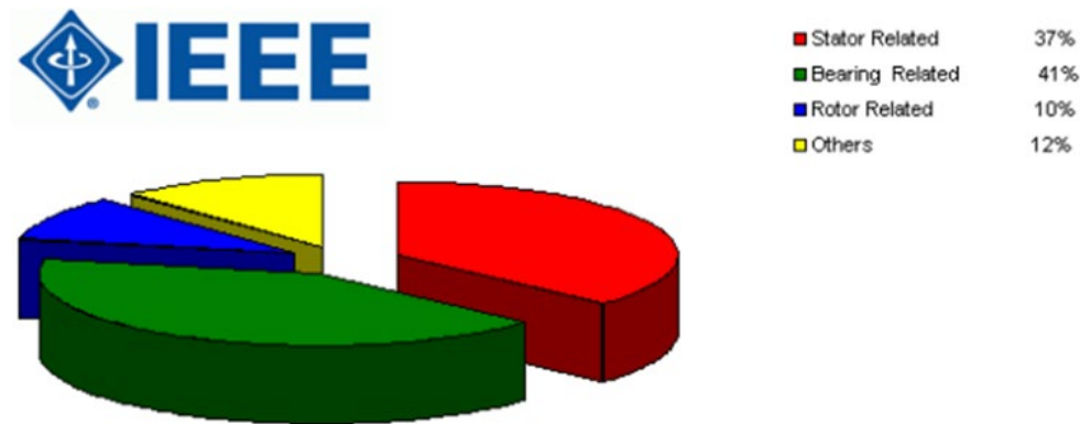
Figure 1: A 1995 IEEE Study on causes of motor failure show stator and rotor issues account for 47 %
