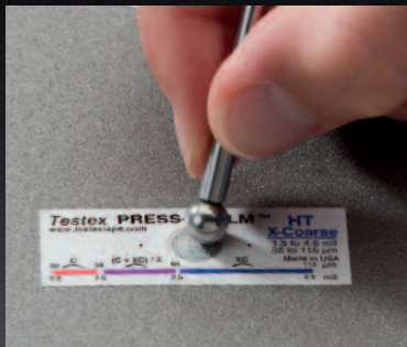
For use with Testex™ Press-O-Film™ Replica Tape
