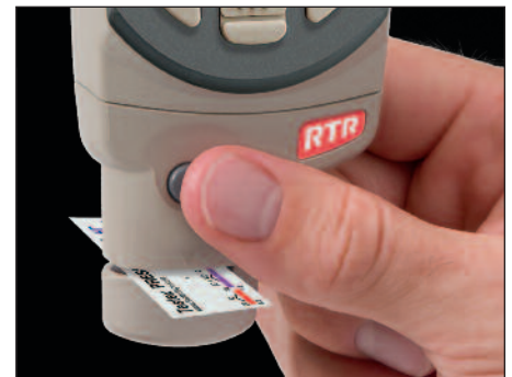
Align probe arrows with tape positioning dots
