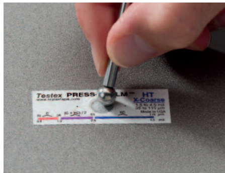
Stainless Steel Burnishing Tool ensures consistency
