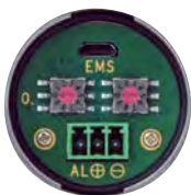
Thermalert 4.0 supports 2-wire loop
